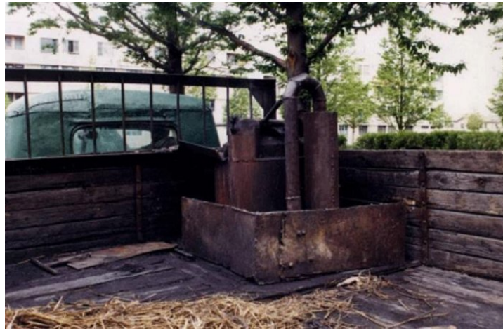
DPRK truck powered by a coal (and/or biomass) gasifier. Source: Nautilus Institute
